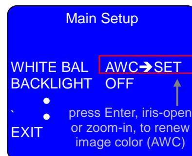
**Manual:** To adjust color preference manually. Manual setting is let you fix the color temperature, which can be good for indoor and static environment. If the lighting is tungsten or alike (more natural), try to add more blue or
