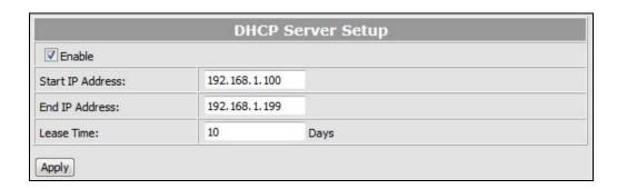
**Enable:** Click the checkbox to enable or disable DHCP Server function. When the function is activated, the NVR can be treated as the DHCP server. The NVR will assign or distribute one of the IP address which is according to the setup IP address range (start and end IP Address.) to the connecting IP camera or video server (these devices must enable DHCP function as well).
