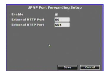
**Enable:** Click the checkbox to enable or disable the "UPnP Port Forwarding" function. This function provides an easy way to configure the NAT (Network Address Translation) in router. If the router equips "UPnP Port Forwarding" function too, the NVR will ask the router to open the "External HTTP Port" and "External RTSP Port" for the NVR automatically. Therefore, you don't need to configure the Port Forwarding
