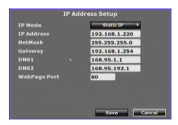
IP Mode: Click the pull-down list to change the IP mode to Static IP or DHCP.
