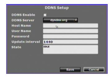
**DDNS Enable:** Click the checkbox to enable or disable the DDNS function.
