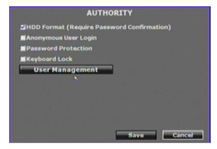
**HDD Format:** Click the checkbox to enable or disable the authority of HDD Format function. If enable this function, the user has to input password while performing HDD format.
