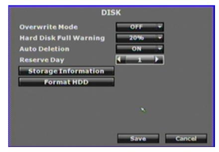
Overwrite Mode: Click the pull-down list to enable or disable overwrite function.
