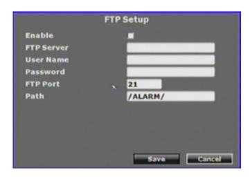
**Enable:** Click the checkbox to select which event should send message to FTP server when it is triggered.
