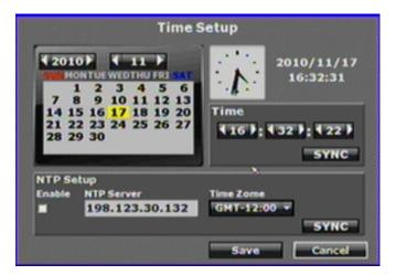
**[SYNC] button in "Time" block:** Click this button can adjust and synchronize the time of NVR as the system time of PC.
