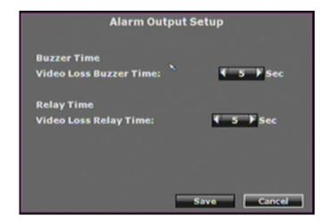
**Video Loss Buzzer Time:** Click ◀ or ▶ to change the buzzer time when video loss is detected. The available value is from 5~99 seconds.
