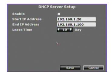
**Enable:** Click the checkbox to enable or disable DHCP Server function. When the function is activated, the NVR can be treated as the DHCP server. The NVR will assign or distribute one of the IP address which is according to the setup IP address range (start and end IP Address.) to the connecting IP camera or video server (these devices must enable DHCP function as well).
