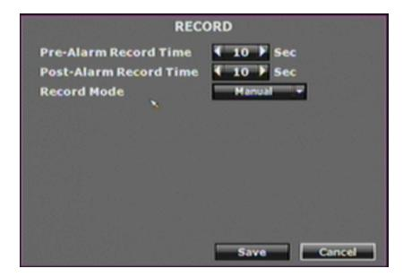
**Pre-Alarm Record Time:** Click ◀ or ▶ to change the recording time of pre-alarm. The available value is from 0~30 seconds.
