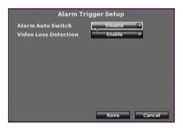
**Alarm Auto Switch:** Click the pull-down list to change the display mode when an alarm is triggered. When the alarm is triggered, the screen will switch to full screen, split screen or disable.
