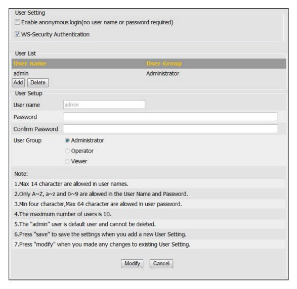
The user configuration page allows the Network Camera to have multiple users and profiles to access the Network Camera.
