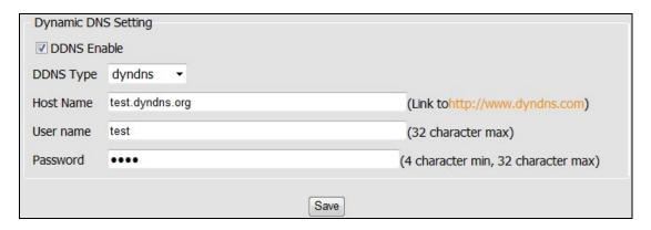
The DDNS (Dynamic Domain Name Service) feature allows users to access the Network Camera without the need of remembering the IP address, but rather using a name.
