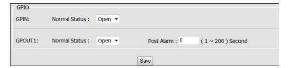
This page is used to configure normal circuit status of Digital Input and Digital Output.
