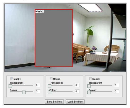
Sets a privacy masking on the selected area; a maximum of 3 privacy masks are allowed. To enable the mask, make a checkmark on the box for enabling it, and after marking the area using the mouse, click on **[Save Settings]** button to make the changes permanent.
