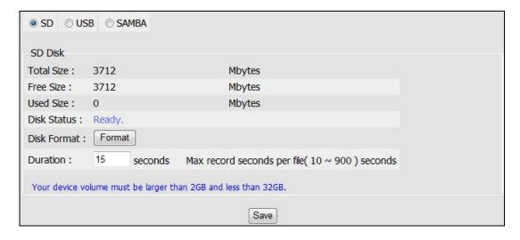
Displays information on the Micro-SD Card inserted in the network camera.
