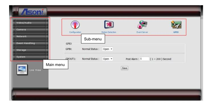
To open the page for configure, click the button on "Main menu" area on the left side, and then click the button on "Sub-menu" on the top side. Refer to the related chapter to configure the camera.
