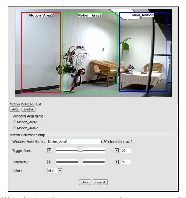
Video motion detection is used to generate an alarm whenever movement occurs in the video image.
