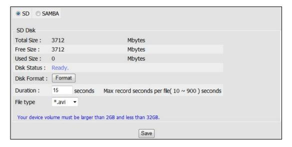
Displays information on the Micro-SD Card inserted in the network camera.
