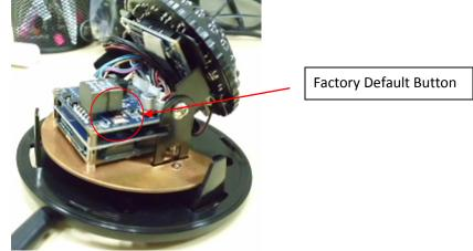
2. Use a wire to insert one end into "Default" and one of the "GND" pin (which are the Pin 5 and Pin 6).
