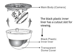
Reinstall the dome cover and the main body by turning the dome clockwise until it locks in place.
