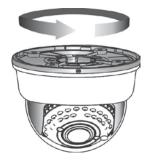
The dome comes with a black plastic inner liner placed within the dome cover. Therefore, after replacing the dome cover rotate the liner so that the cutout slot (hole for viewing) is in the correct position and not blocking the camera lens.
