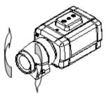
**<u>Note</u>**: it is required get connected to the Network Camera prior to adjust the focus.
